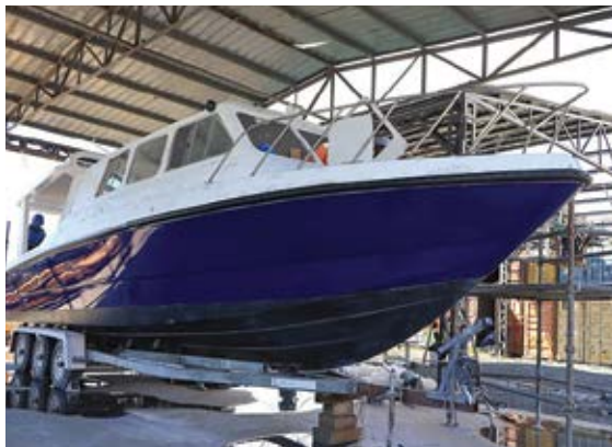
A Fibreglass boat under construction at the Kenya Shipyards Limited at the Mombasa shipyard.
