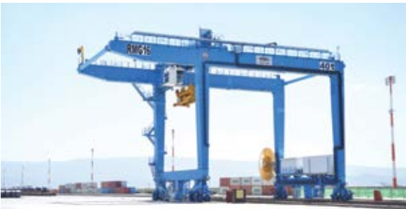
1. KRA Commissioner General Humphrey Wattanga (2nd right) and South Sudan's William Kuol (centre) during an inspection tour of the Naivasha ICD. 2. A rail mounted gantry crane at Naivasha ICD used for loading and offloading containers onto SGR and MGR trains. PHOTO: ERASTUS GICHOHI
