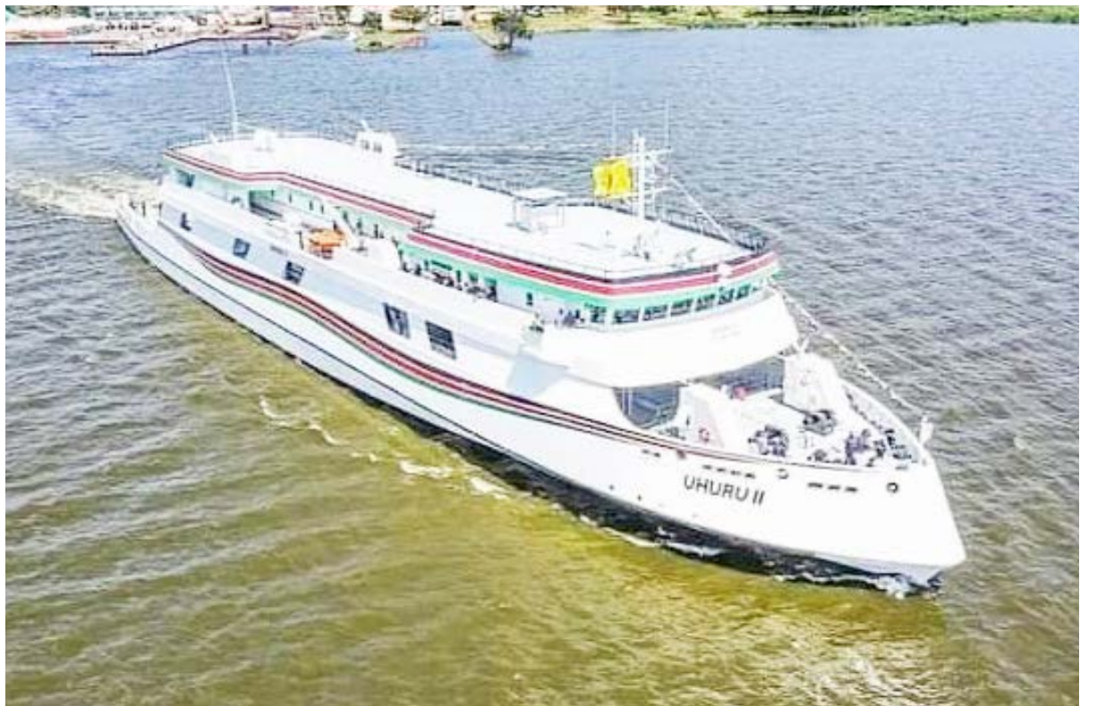
The Sh 2.4 billion MV Uhuru II was assembled locally by Kenya Shipyards Limited (KSL). The 100m vessel has a capacity of 2 million litres of crude oil per trip and 1,800 tons.
