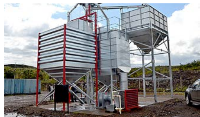
A steam powered grain dryer at Menengai Crater in Nakuru. The first of its kind in Kenya and the region has a capacity of drying 20 tonnes of cereals per day.
