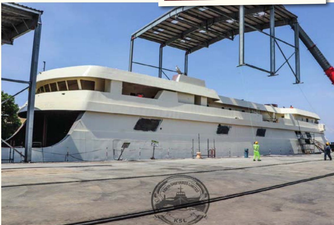
MV Uhuru II is currently in its final stages of construction at the Kisumu Shipyard. The ferry can carry up to 22 wagons and over two million wet or dry cargo per trip. MV Uhuru II is expected to enhance maritime transport in the lake-basin region and facilitate cross-border trade in the Eastern Africa region. PHOTO: KSL
