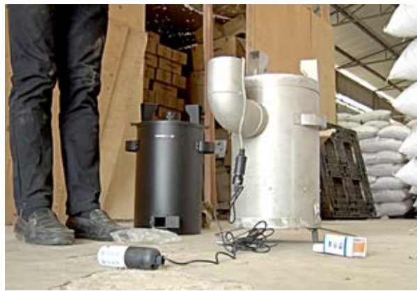
A thermo-electric jiko that uses pellets to produce heat for cooking while at the same time produces energy to power light bulbs and charge phones,
