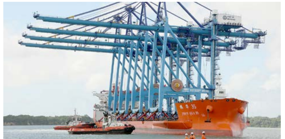
Ship-to-Shore gantry crane. The Port of Lamu has received three such cranes.
