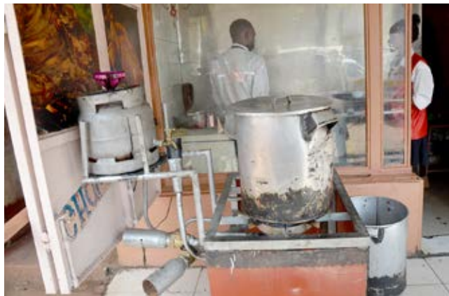
A complete version of old engine oil stove at the Choma Zone hotel in Nyeri town. A two burner commercial stove retails at Sh 40,000 and it requires three litres of used engine oil in a day to function.
