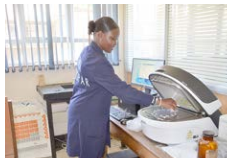
A chemical analyst at Chemistry Lab using an XRF machine to conduct multiple simultaneous tests for minerals on rock samples.
