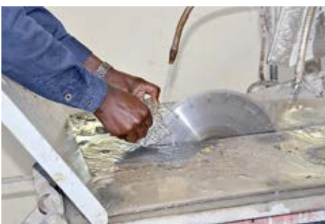
A rock sample being sliced for extraction of a sample for examination under a petrographic microscope.
