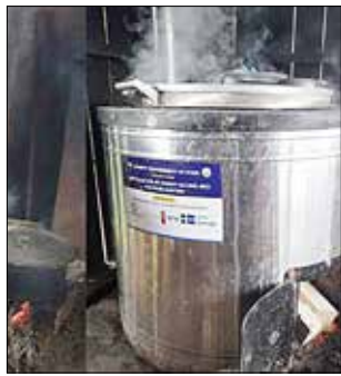
An energy conserving cooker (right) and a traditional three stone hearth to the far right. (Photo: Courtesy)
